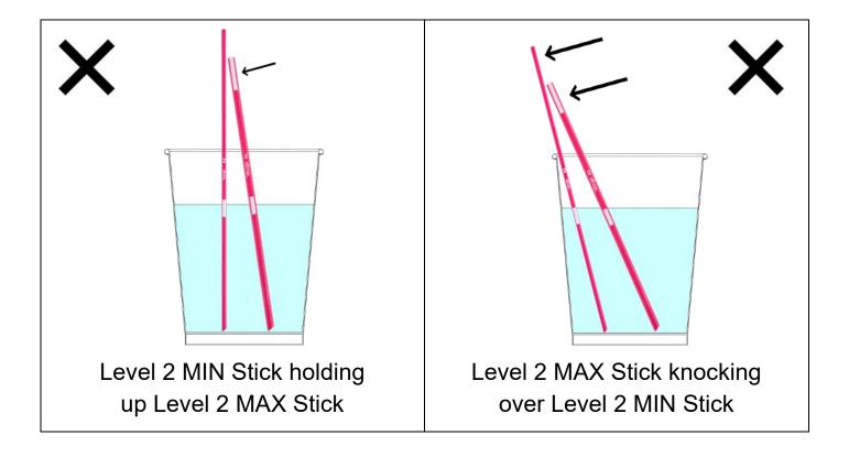
If an unexpected result occurs, for instance a stick falls quicker than expected, it is recommended to perform the test again making sure the stick starts from a vertical position. You might find it easier to ensure the stick is vertical if you use one stick at a time rather than both Sticks together.
