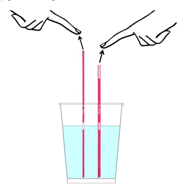
To get a correct result, it is very important to release the sticks from a vertical position. Failure to do so can cause an incorrect result as a stick might fall more quickly than it would if starting from a vertical position. You might find it easier to ensure the stick is vertical if you use one stick at a time rather than both sticks together.
